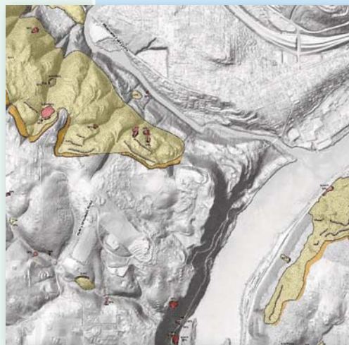
This portion of the Canby Quadrangle Landslide Inventory Map shows existing landslides in West Linn (left) and Oregon City (right).
