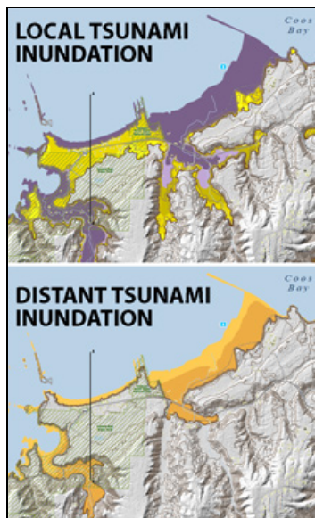
Portions of DOGAMI TIM-Coos-08, Charleston – Cape Arago maps, showing modeled tsunami inundation in the Sunset Bay State Park area.
